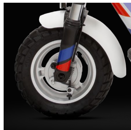
10" Off-Road tyres with air chamber
